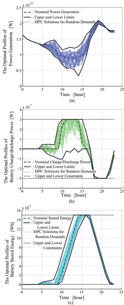
Fig. 4. (a) The Optimal Profiles of Power Generation, (b) The Optimal Profiles of Battery Charge/Discharge Power, (c) The Optimal Profiles of Battery Stored Energy
