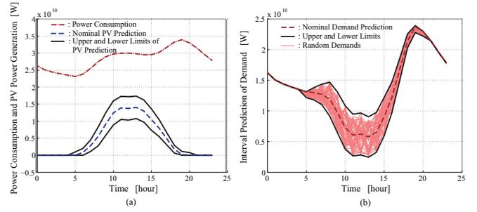
Fig. 3. (a) Power consumption and PV power prediction, (b) Interval Prediction of demand
